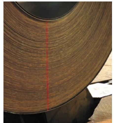
During measurement a laser line illuminates the head site of a coil
