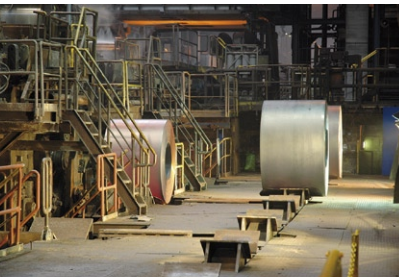
Transportation of coils at hotstrip mill (ThyssenKrupp Steel AG, WBW Bochum, Germany)
